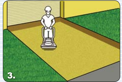
3. Compact the sand to 100mm thickness
