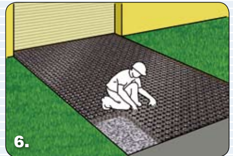
6. Lay down 52mm Gravel Cell®
