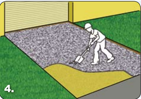
4. Lay down mixture of sand & topsoil (growing Media) to 100mm.
