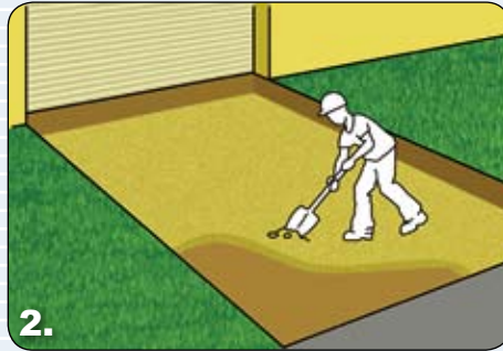
2. Lay a 100mm layer of washed coarse river sand.
