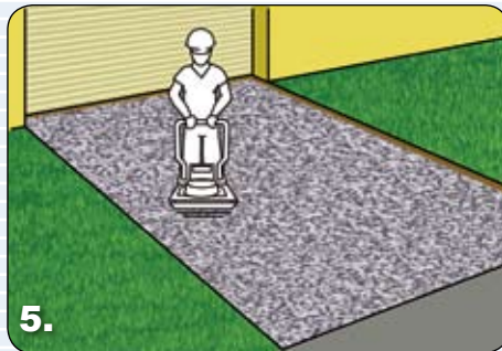
5. Compact the gravel to 100mm
