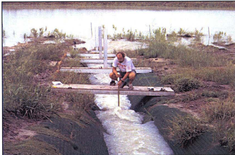
Flow test at TTI's "real world" outdoor test flume.
