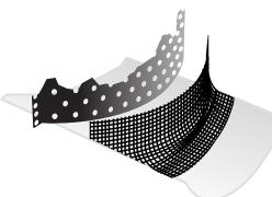
Place Plastic netting on Trash Guard® as Shown. Bend and conform plastic netting to shape of Trash Grard® and Drain with 90 degrees bend away from Trash Guard® to allow for assembly to bottom of drain. Cut plastic netting to conform to Trash Guard® and shape of drain.
