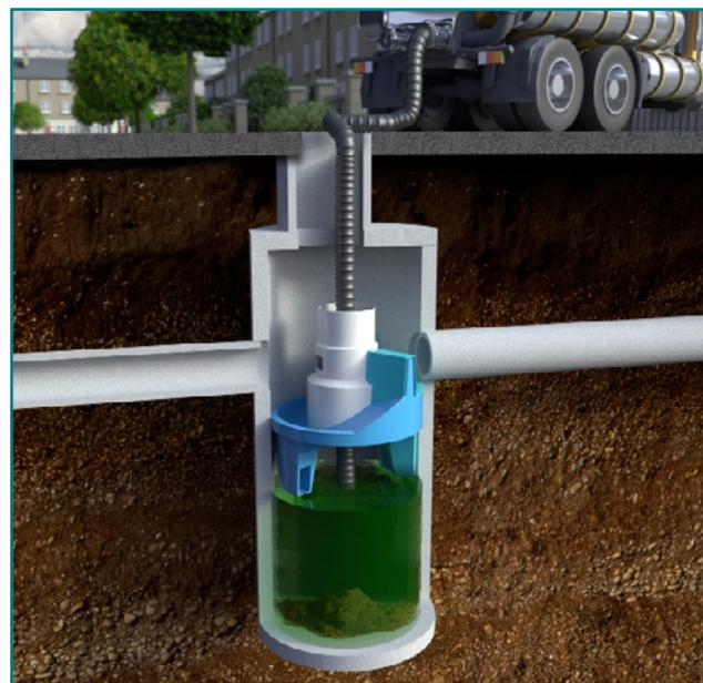
Fig 3. Maintenance is done with a vector truck
